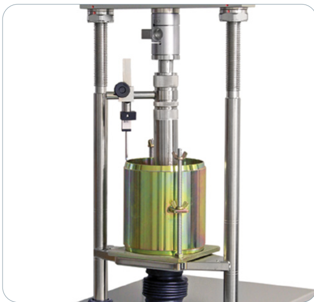
Set for performing CBR tests (accessories have to be ordered separately).
