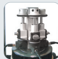
Elastic Modulus on mortar and Cement
