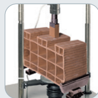
Punching and bending test on clay and concrete blocks for flooring
