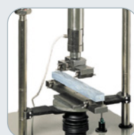
Flexural test on soil - cement specimens
