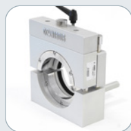
Interlayer bonding / Shear bond Test (Leutner)
