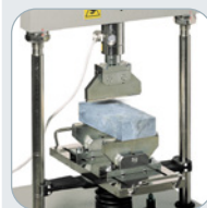
Modulus of rupture of natural building stones
