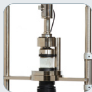
Compression on low strength mortar mixes
